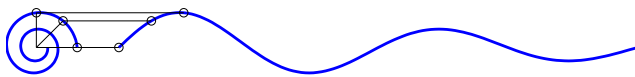
Figure 24.5: A single phasor plotted as a damped two dimensional rotation \mathbf{h}_{t+1} = \gamma \mathbf{R}_\theta \mathbf{h}_t with a damping factor 0 < \gamma < 1 . By taking a projection onto the y axis, the phasor generates a damped sinusoid.
