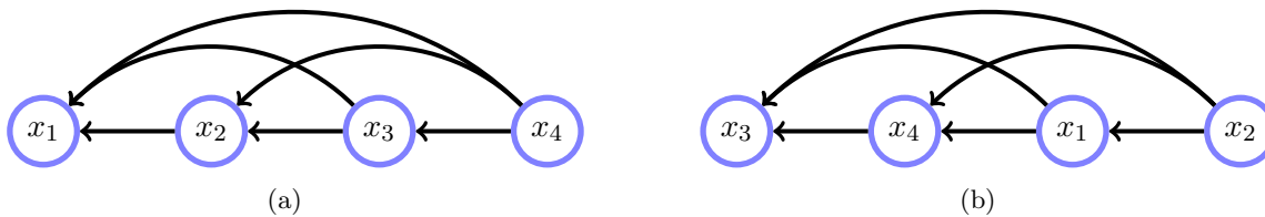
Figure 3.3: Two BNs for a 4 variable distribution. Both graphs (a) and (b) represent the same distribution p(x_1, x_2, x_3, x_4) . Strictly speaking they represent the same (lack of) independence assumptions – the graphs say nothing about the content of the CPTs. The extension of this ‘cascade’ to many variables is clear and always results in a Directed Acyclic Graph.
